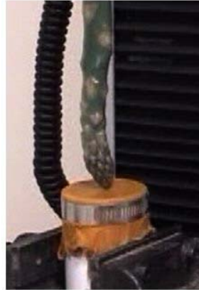
Figure 7 - Photographs of Alternative Asparagus Pre- and Post-Buckle
