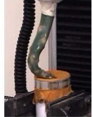
Figure 7 - Photographs of Alternative Asparagus Pre- and Post-Buckle
